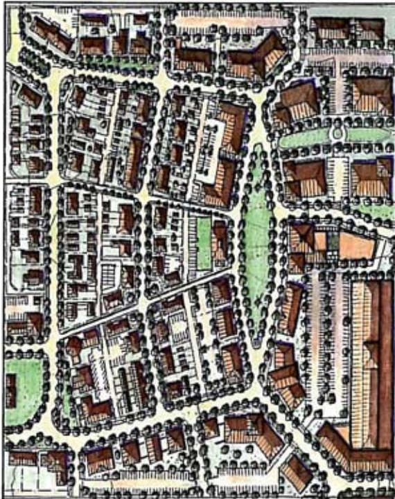
The Hellgate Meadows site plan demonstrates the concept of high density at town center and diminished density toward the edges. © Oliver Kuehne/HDR
